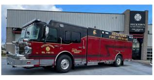
delivery of our new pumper rescue truck, 5341. This truck will serve a dual purpose as our primary rescue unit for auto accidents and other rescues as well as being a front line pumper with a 1750-gallon per minute pump and a 1,000-gallon water tank. The anticipated service life of this truck is twenty to thirty years. Lower Nazareth Township was instrumental in providing funding and securing grants to cover the cost of this new apparatus.
